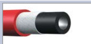
Non wire, braided hose consists of an extruded tube and cover with layers of braided synthetic cord.
