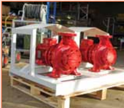
FAST FILL WATER TANKER - PUMP SETS
