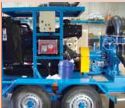
TRAILER MOUNTED DIESEL PUMP SET 225HP
